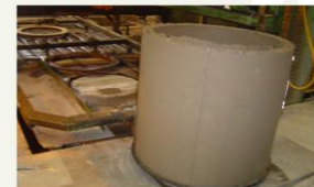
Picture (23): A manhole is pushed by the cross pusher
