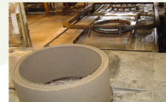
Picture (24): Short length manhole waiting in the WIP area for some finishing works
