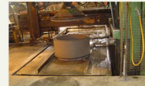
Picture (21): The cross pusher is pushing the manhole off
