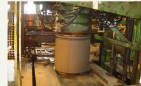
Picture (22): The manhole is waiting the cross pusher
